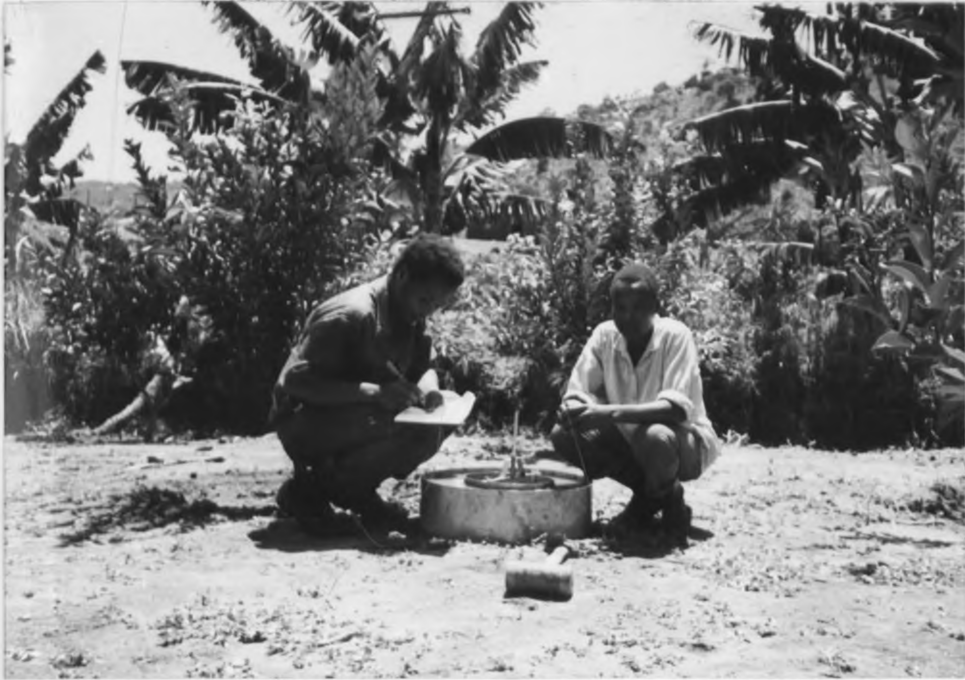
Plate 3.1. Measurement of instantaneous infiltration rate at Experimental Site.
