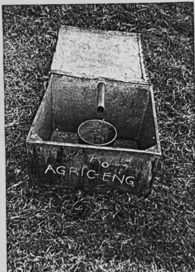
Plate 1. Storage tank with container for small storm.
