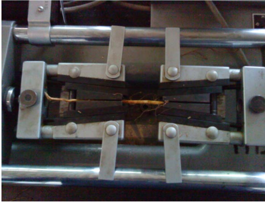
Fig. 4: Clamping of the roots using wedge grips
