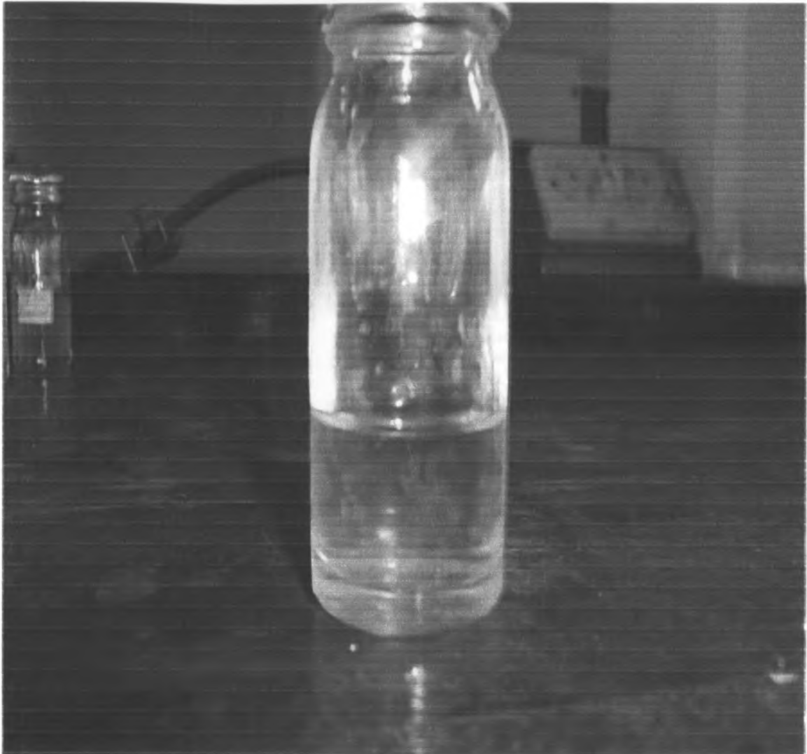
Figure 3-6: Pure bio-diesel (B-100) after being washed (soap content-75ppm, density 0.89 \text{ g cm}^{-3} , pH 6.9)
