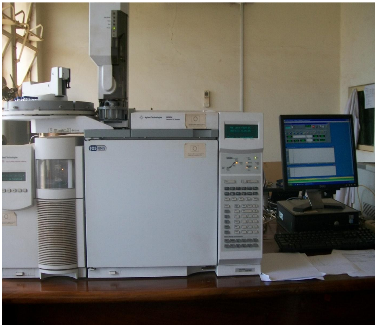
Figure 66: Agilent Technologies 6890N Network Gas Chromatograph used in the GC-MS analysis.
