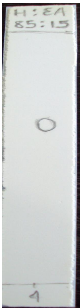
Figure 64: TLC of compound 4P developed using hexane/ethyl acetate (85:15) mixture.
