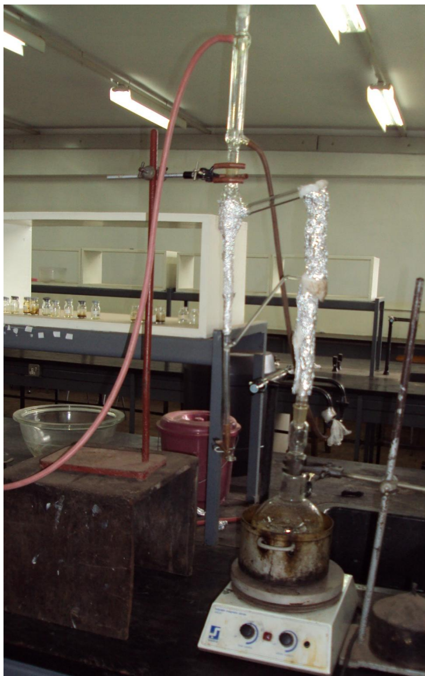
Figure 65: The set up for Clevenger distillation.
