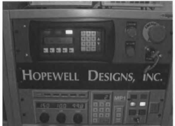
(d) The MPI control console for settings of kilovoltage (kV) and current (mA)
