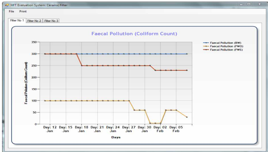
Figure 4.3: comparing the faecal contamination levels for raw and filtered water
