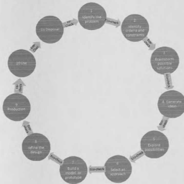
Plate No. 4.9: Cradle to cradle product life cycle Eco-check proposed by the researcher
