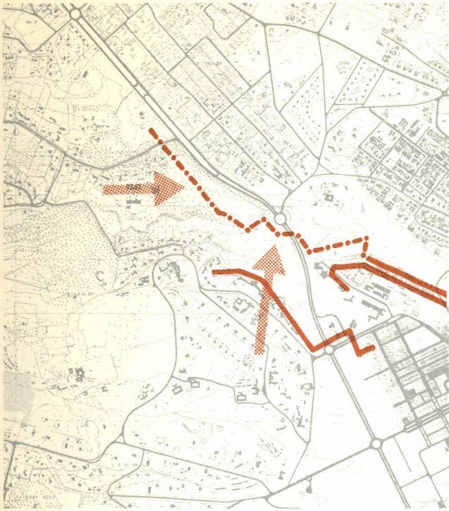
SEWAGE DISPOSAL 1:30,000 Full line: Existing Sewers Dotted line: Planned sewer Arrows indicate main direction of sewers for U.C.N. development.
