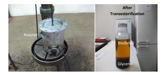
Fig 3.5: Reactor during transesterification and separation of Biodiesel and Glycerol.
