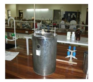
Fig 3.8: Constant –volume bomb calorimeter
