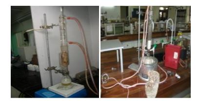
Fig 3.4: Soxhlet apparatus for solvent extraction.
