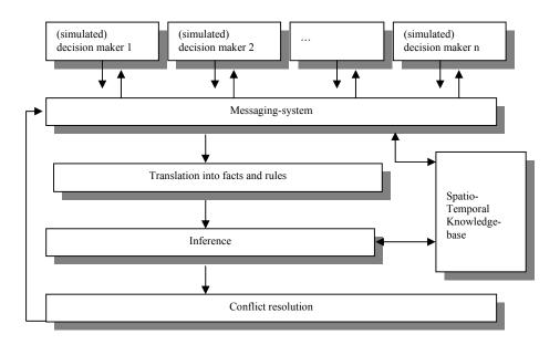
Figure 1: Principle of the TIS Architecture
