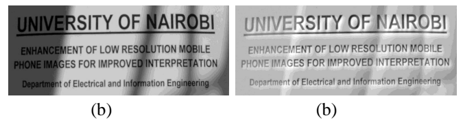
Fig. 15: Shadow removal using SSR. (a) Input image (b) SSR enhanced image.
