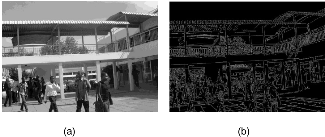
Figure 7.14: Sobel filtering. (a) Input image. (b) Output image.
