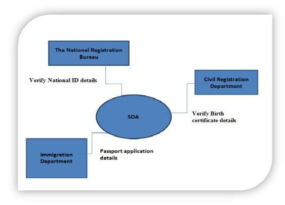
Fig. 4.1 SOA Component Diagram
