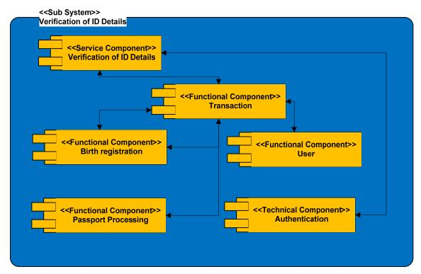
Fig. 4.3 ID Verification subsystem.
