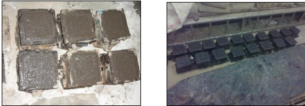
Plate 3.6: Preparation of Concrete Specimens for Strength Tests
