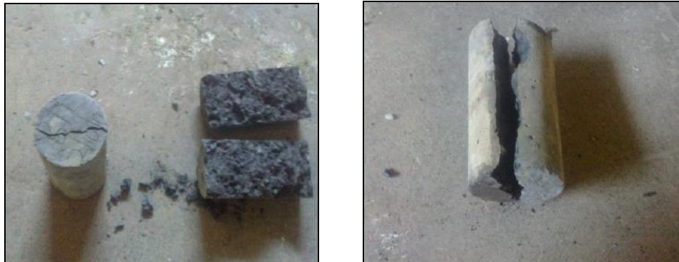
Plate 3.10: Concrete Cylinder Specimen Mode of Failure
