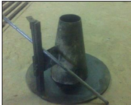
Plate 3.4: Slump Test Apparatus
