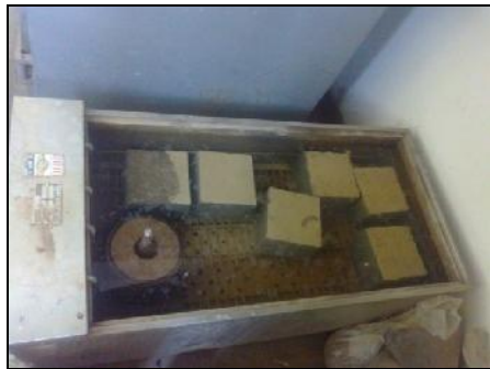
Plate 3.7: Curing of Concrete Test Specimens
