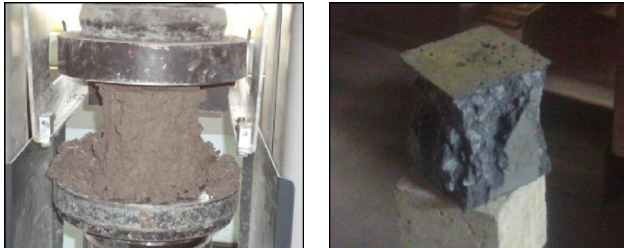
Plate 3.9: Concrete Cube Specimen Mode of Failure
