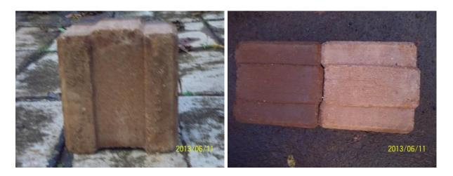
Plate 5 & 6: Standard Hydraform Bock (Sample of Interlocking Stabilised Soil Block)
