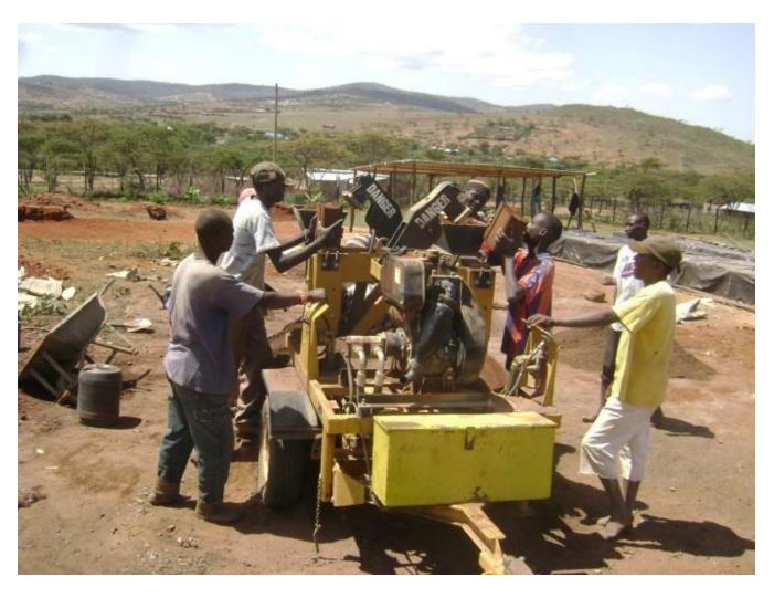
**Plate8: ISSBs production in progress**
