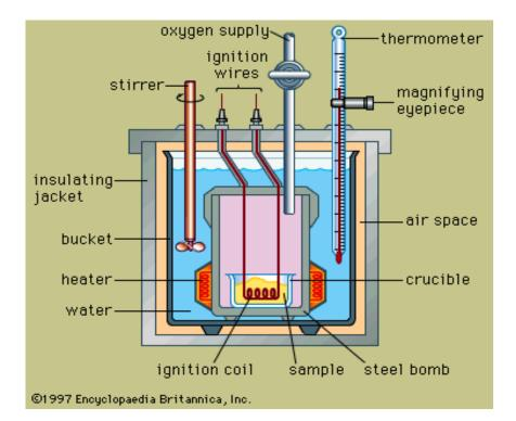
Bomb Calorimeter-instrument used to measure calorific value of fuels
