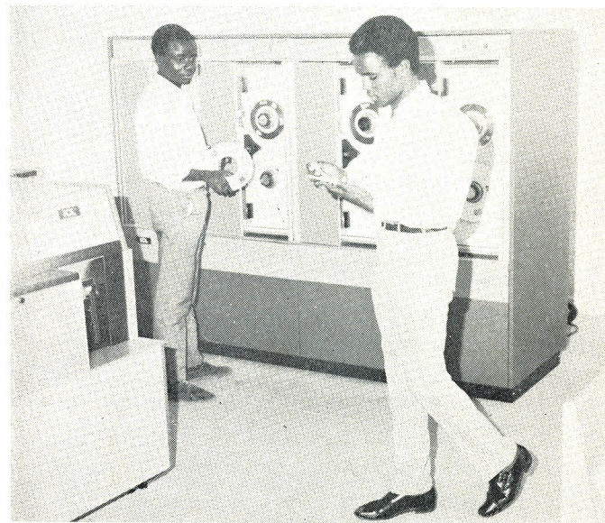
The computer tape decks, where information is recorded on tape for storage. In the foreground is Mr. David Mukuriah, a computer operator.
