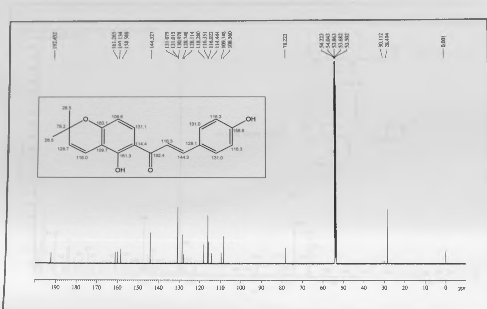
Appendix 26B: ^{13}\text{C} -NMR spectrum of 4-hydroxylonchocarpin (239), \text{CD}_2\text{Cl}_2 , 150 MHz
