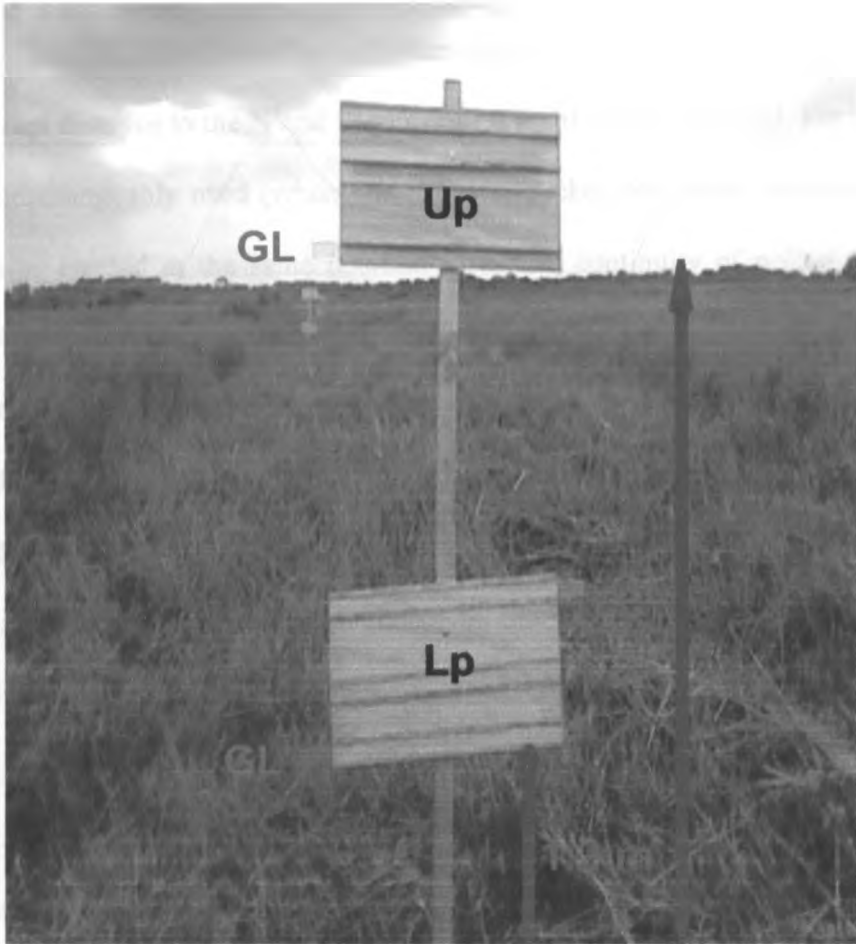
Plate 3.2: Pollen traps; upper (Up) placed at a height of 1.8 m and lower (Lp) placed at a height of 1.2 m, and fixed the glass slides (GL).
