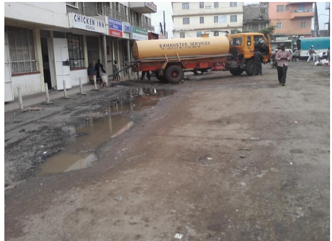
Fig 10 Appendix 1D: Exhauster emptying septic tank at Crystal Plaza in Ongata Rongai
