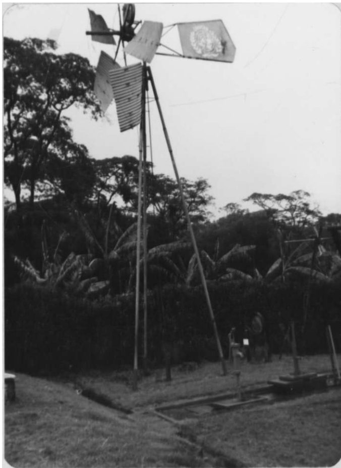
Plate 8: A wind mill used to pump water from wells dams to homesteads. It reduces the cost of pumping water.
