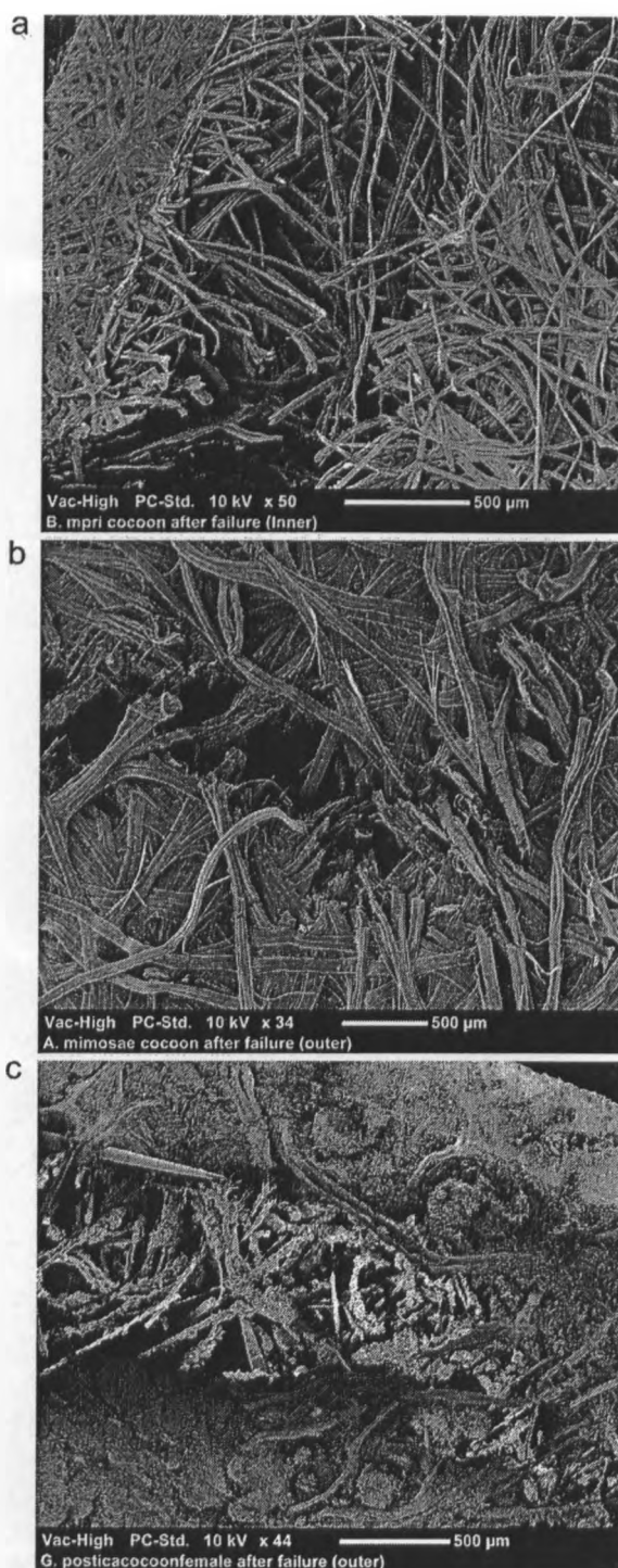
Figure 2. SEM micrographs of fracture surfaces of cocoon shells after tensile failure.
