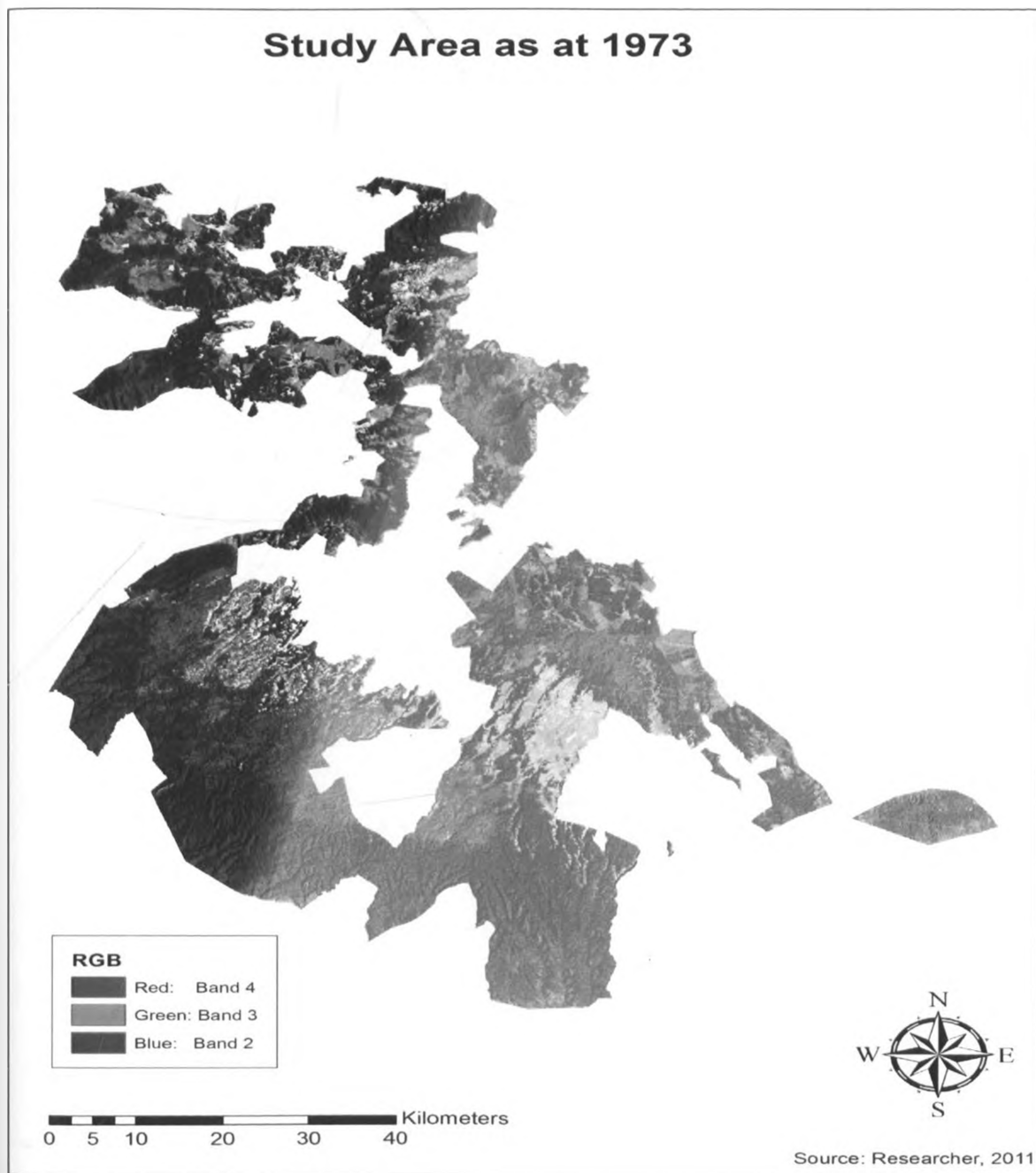
Figure 6.1a: NIR false colour composite of bands 4, 3 and 2 for the study area as at 1973
