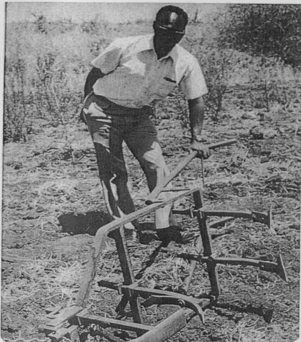
Figure 3.7 Two A-shares in the rear and one chisel share in the front moulded on the Ariana tool bar
