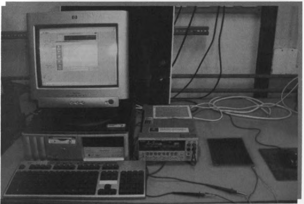
Figure 3.3: Photograph of the DSSM's dark J - V characterization experiment set-up [The DSSM was not covered when taking this photograph for purposes of visibility. It was however covered during the actual dark J - V characterization].
