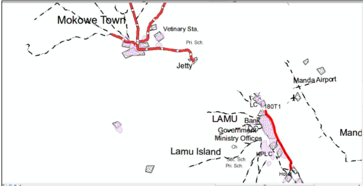
Figure 33: Building generalization by use of delineate built-up area tool
