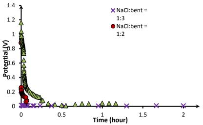
Figure 12: A plot of potential versus time for polyaniline modified electrode in NaCl:Bentonite (mass/mass) - 1:3, 1:2, and 1:1.
