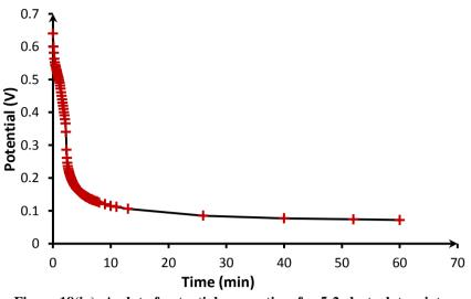
Figure 18(iv): A plot of potential versus time for 5:2 electrolyte mixture.
