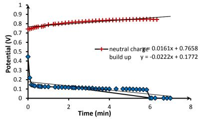
Figure 27: A plot of potential versus time for discharge/re-charge. The electrolyte mixture is hydrocarbon gel:bentonite = 3:1.
