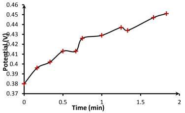
Figure 26: A plot of potential versus time for stabilization of neutral voltage. The electrolyte mixture is NaCl:bentonite 1:3.
