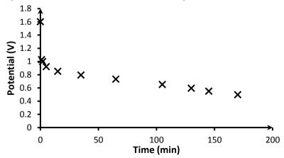
Figure 4: A plot of potential (V) versus time for bare carbon electrode.
