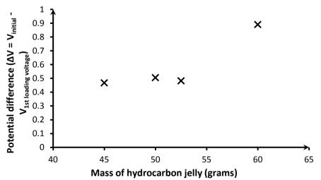
Figure 17: A plot of potential difference ( $\Delta E$ ) versus mass of hydrocarbon gel (grams). The electrolyte mixture of hydrocarbon gel: bentonite 3:1, 3.5:1, 4:1, 5:2. Amount of NaCl is equal to that of bentonite.
