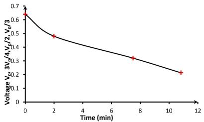
Figure 19(i): A plot of potential (V<sub>0</sub>, 3V<sub>0</sub>/4, V<sub>0</sub>/2, V<sub>0</sub>/3) versus time (min). The electrolyte mixture of petroleum jelly: bentonite 3:1. Amount of NaCl is equal to that of bentonite.
