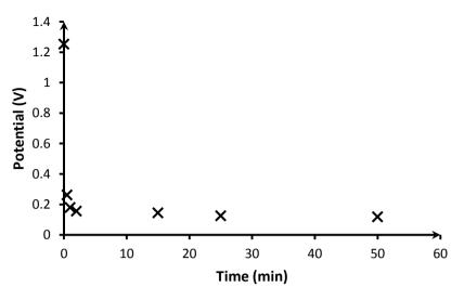
Figure 5: A plot of potential (V) versus time for polyaniline modified carbon electrode in solution containing 0.1 M aniline and 0.5 M H<sub>2</sub>SO<sub>4</sub>.
