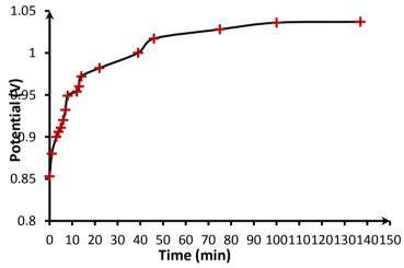
Figure 20: A plot of potential versus time for stabilization of neutral voltage. The electrolyte mixture of hydrocarbon gel: bentonite is 4:1.
