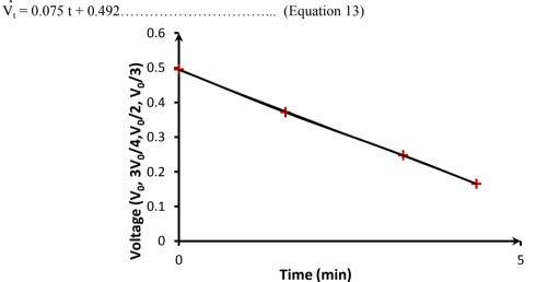
Figure 24: A plot of potential  $(V_0, 3V_0/4, V_0/2, V_0/3)$  versus time (min). The electrolyte mixture of NaCl:bentonite 1:1.
