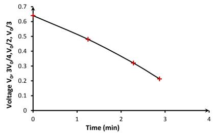
Figure 19 (ii): A plot of potential (V<sub>0</sub>, 3V<sub>0</sub>/4, V<sub>0</sub>/2, V<sub>0</sub>/3) versus time (min). The electrolyte mixture of hydrocarbon gel: bentonite 5:2. Amount of NaCl is equal to that of bentonite.
