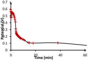
Figure 15 (i): A plot of potential versus time. The electrolyte mixture of hydrocarbon gel :bentonite (1:1). Same amount of NaCl as the bentonite.
