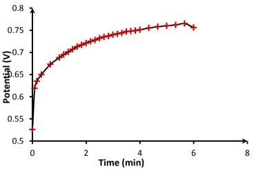
Figure 22: A plot of potential versus time for stabilization of neutral voltage. The electrolyte mixture of NaCl:bentonite 1:1.
