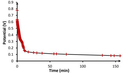
Figure 16: A plot of potential versus time. The electrolyte mixture of hydrocarbon gel: bentonite 2:1. Same amount of NaCl as the bentonite.
