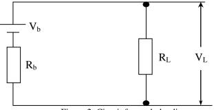
Figure 2: Circuit for study loading.
