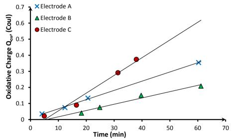
Figure 3: Plot of oxidative charge,  $(Q_{,ox})$  versus time for polyaniline electrodeposited on a bare carbon electrode in solution containing 0.1 M aniline and 0.5 M H<sub>2</sub>SO<sub>4</sub>. The potential range was from – 0.2 to 0.80 V. Scan rate 20 mV/s.
