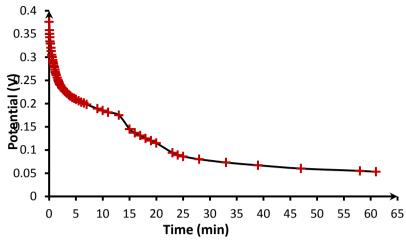
Figure 21: A plot of potential (V) versus time (min). The electrolyte mixture of hydrocarbon gel: bentonite 2:1, and 0.1 M H<sub>2</sub>SO<sub>4</sub>.
