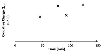
Figure 7: Plot of oxidative charge, (Q<sub>,ox</sub>), versus time for polyaniline electrodeposited on a bare carbon electrode in a solution containing 0.1 M aniline and 0.1 M H<sub>2</sub>SO<sub>4</sub>. The potential range was – 0.2 to 0.80 V at a scan rate of 20 mV/s.
