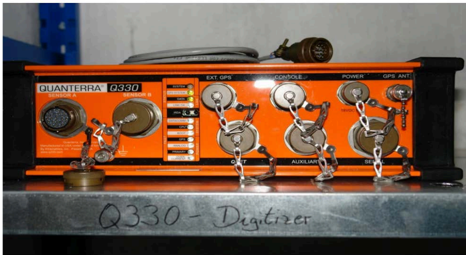
Plate 1-3: The Q330 digitizer which is used at Lodwar station.
