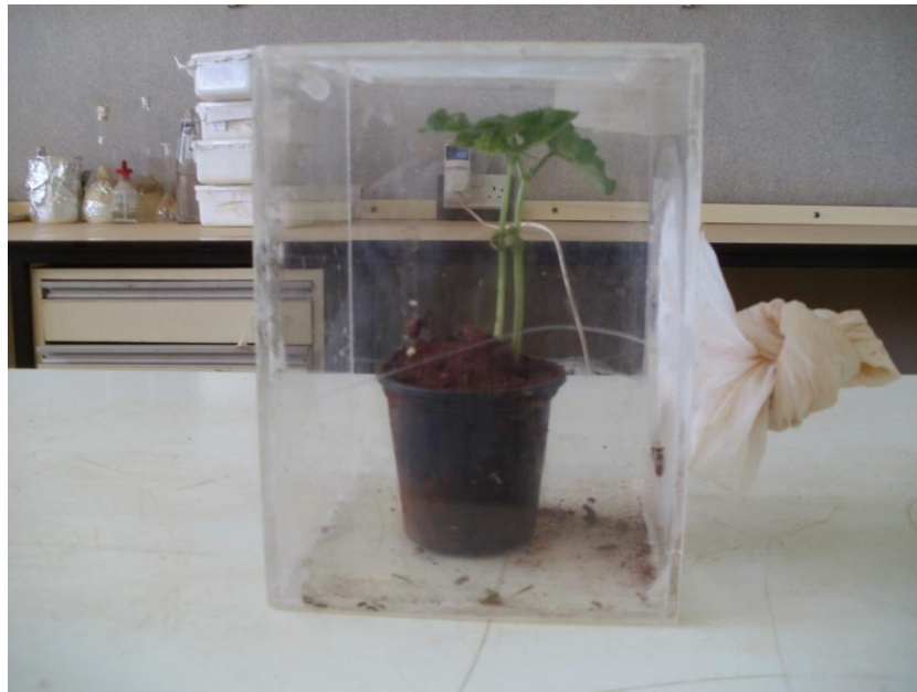
Figure 1: Insect cage for holding a pair of flies with one potted plant
