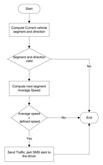
Figure 15: Send Traffic Jam Notification to the Driver Flowchart (Source: Author)
