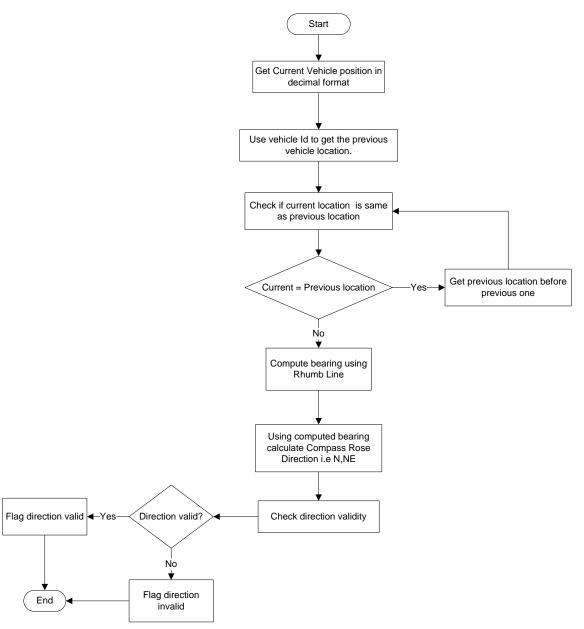
**Vehicle Current Moving Direction Computation Flowchart**
