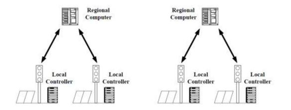
Figure 3 The Physical Architecture of SCATS (Source: Dineen & Cahill, 2001).
