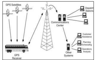
Figure 1 Schematic Display of an AVL System (Source: Casey, et al.,
