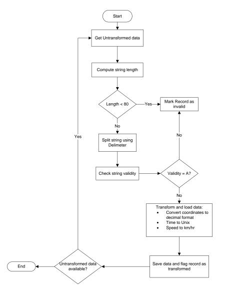
Figure 10: Transform and Load Data Flowchart (Source: Author)
