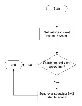
Figure 14: Over-Speeding SMS alert Flowchart (Source: Author)
