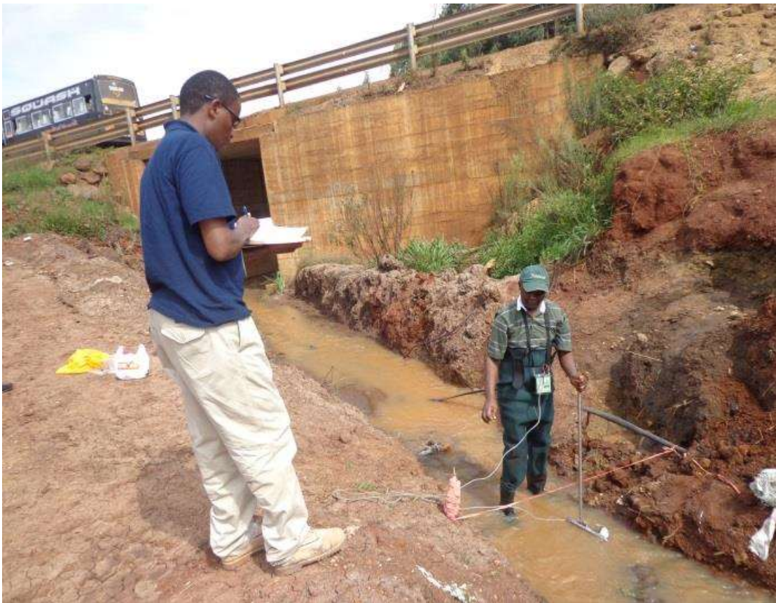
Plate 3.1: Taking discharge measurements using current Meter by wading at Motoine River, Ngong Road Bridge on 17/12/2013.
