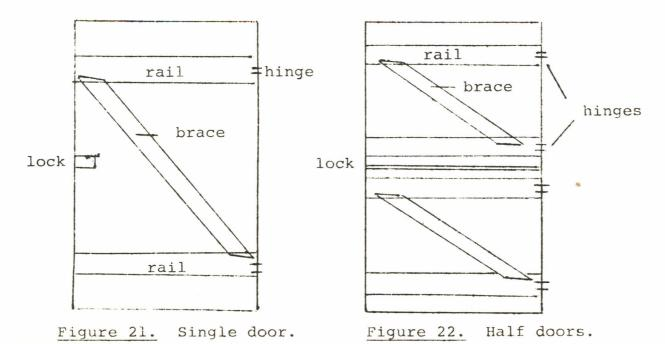
Notice the direction of the braces. They should get support at the hinges. Figure 22 could be a full height door or it may be two half doors, cut horizontally in the middle.
