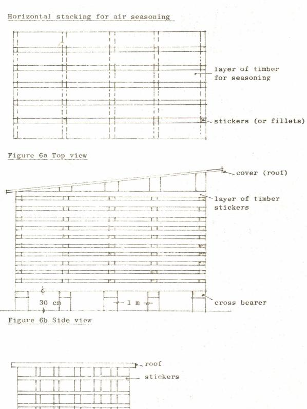
roof stickers timber placed on top for drying. The area under the stack must be kept clear so as to allow air to flow and for drainage.
