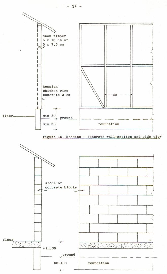
Figure 16. Block wall- section and side view
