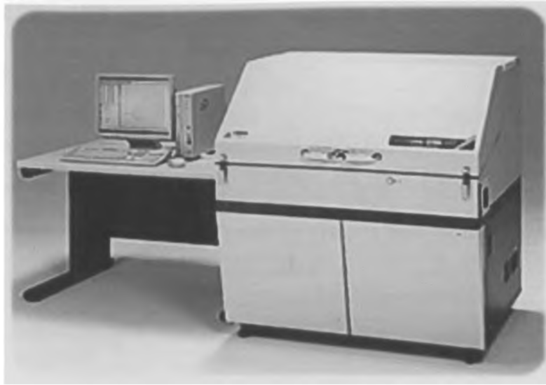
Fig. 4.8: (a) Solid Spec-3700 DUV; UV-VIS-NIR Spectrophotometer interfaced with a microcomputer.
