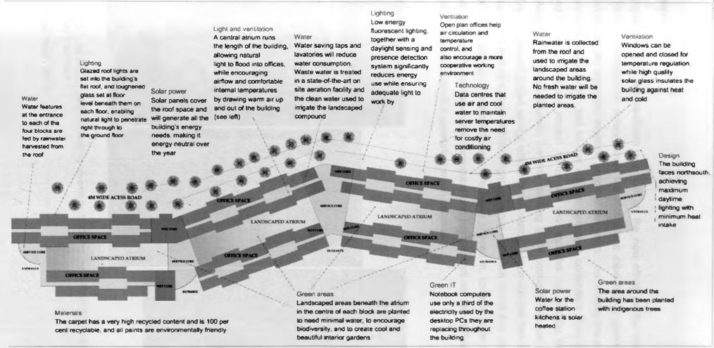
Figure 2.3: Interactive floor plan of the UNEP Building Source: UNEP, (2011) Scale 1/750
