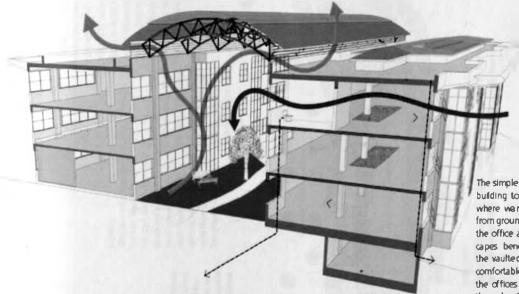
The simple design enables the building to act as a chimney, where warm air is drawn up from ground level and through the office areas, and then escapes beneath the sides of the vaulted roof, maintaining comfortable temperatures in the offices and air circulation throughout the building.
