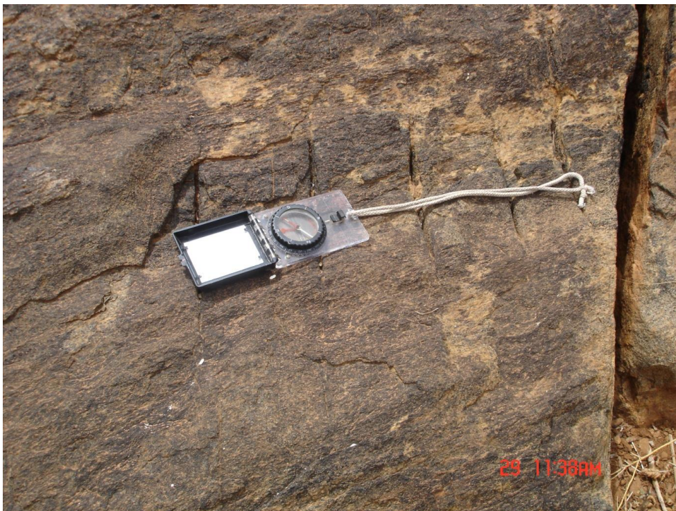
Figure 4.54: Vertical joints trending 212 degrees south west on a Hornblende Gneiss at waypoint 0404434/9767251
