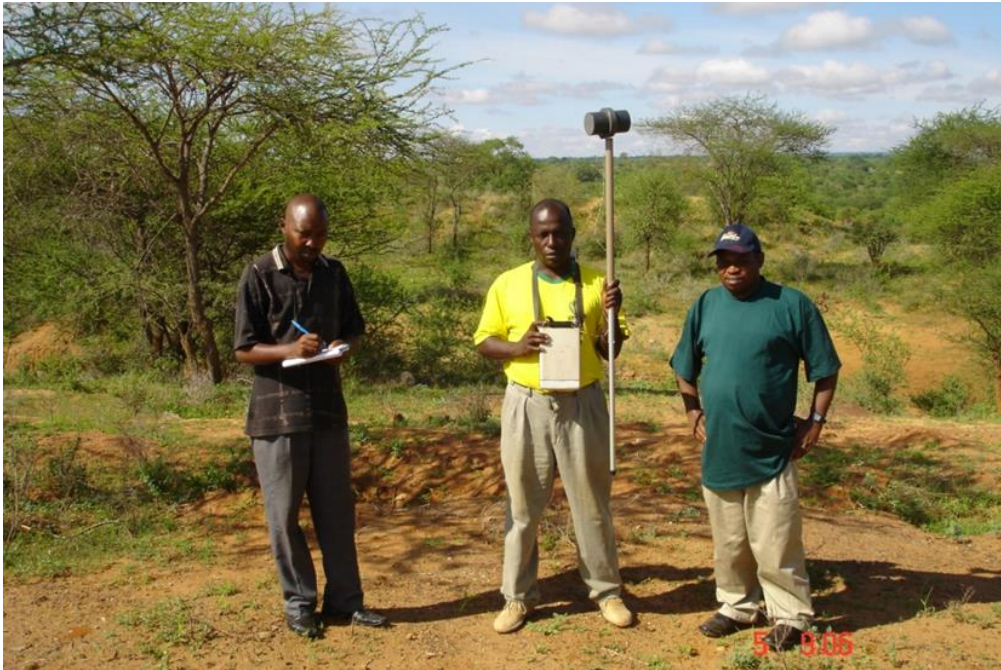
Figure 3.4: Ground Magnetic survey in the project area using Proton precession Magnetometer
