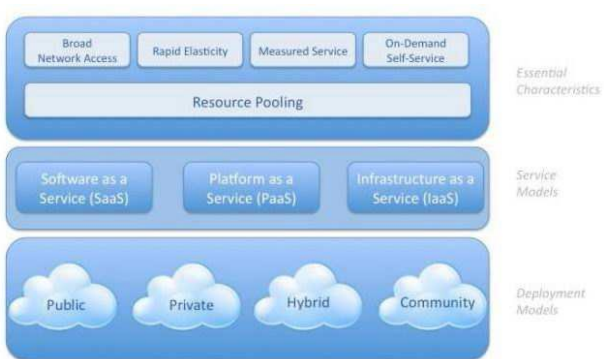
Figure 6 Cloud computing Pictorial Definition: Source- NIST Working Definition of Cloud Computing (cloud alliance 2009)
