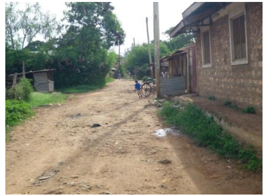
Raising the floor levels of buildings to minimize the effect of flooding.
