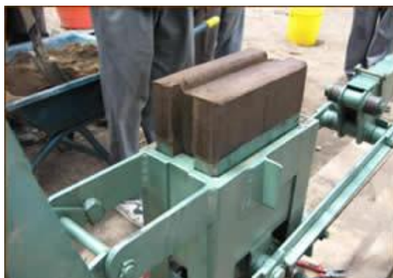
An interlocking stabilised block and the interlocking block maker
