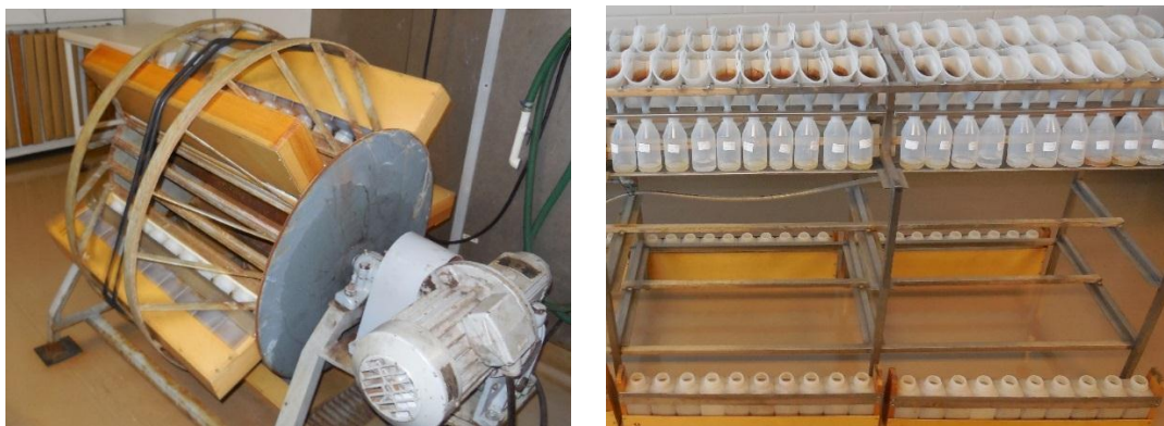
Figure 3.4: Shaking the extraction solution with the sample and filtering the resulting suspension
