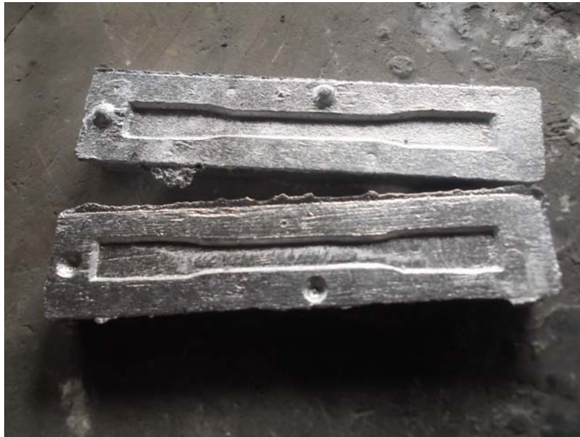
Figure 4.5: The mould after casting showing rough edges.
