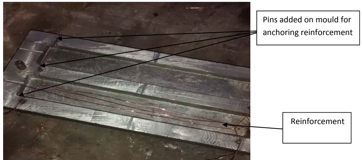
Figure 4.7: Moulds for the three-point bending-test show added reinforcement anchoring pins.
