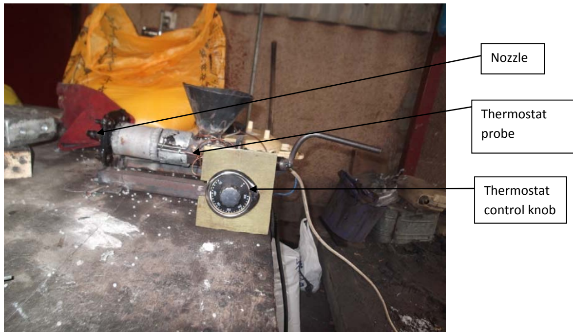
Figure 4.2: The modified injection machine with a nozzle at the outlet, the hopper directly lying on the barrel and with a thermostat for temperature control.
