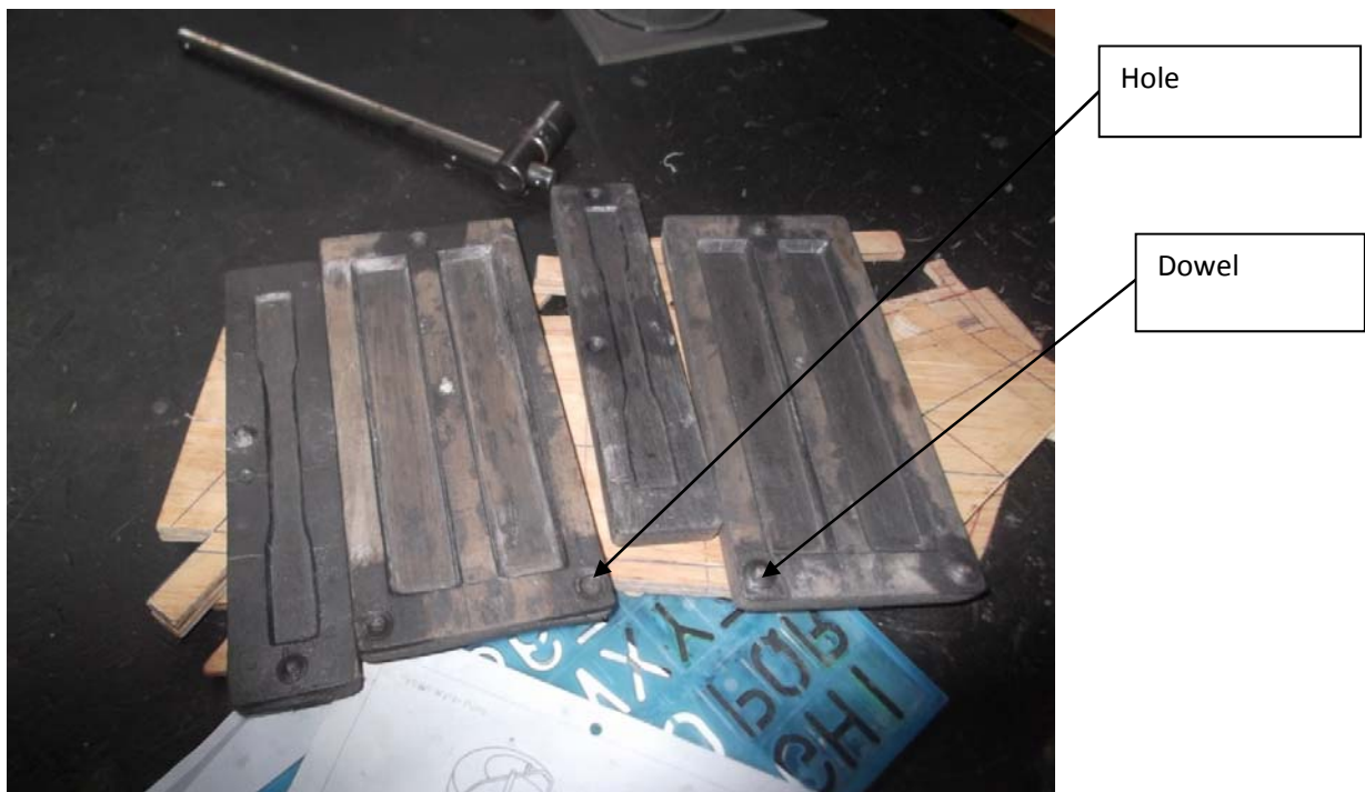
Figure 4.4: The wooden patterns sprinkled with graphite.
