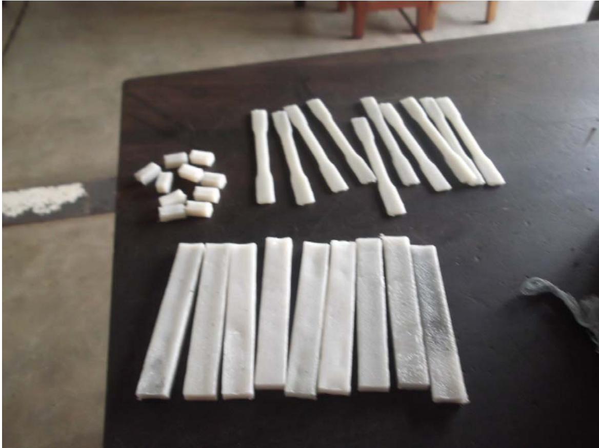
Figure 4.9: Test specimens: On top left are samples for compression test, samples for tensile test on top right and for the three-point bending test at the bottom of the picture.
