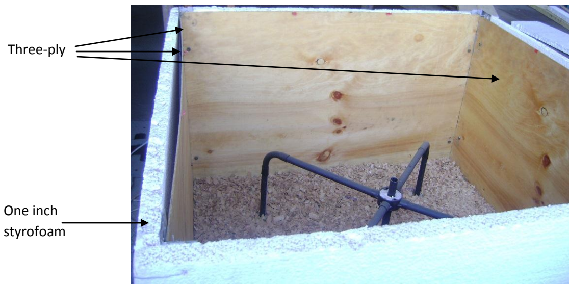
Figure 3.7 Brooder walls – three ply and styrofoam
