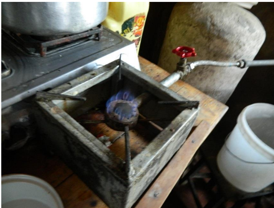
Plate 4.7: Single burner cooking stove is a locally modified biogas burner. It is equipped with medium nozzle and adjuster to control the gas flow. (Source: Field Data, 2014)
