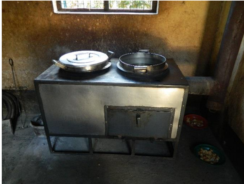
Plate 4.5: Three Chamber Stove is a firewood stove which is available in different sizes. It is adopted from institutional jikos. A chimney is fitted on the outside to emit smoke, wood is feed on the bottom of the stove then lit before placing the pot. Extra wood is feed through the inlet. (Source: Field Data, 2014)
