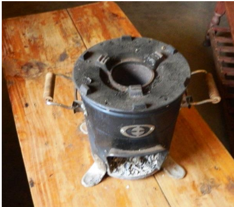
Plate 4.2: Envirofit Stove (M 5000) is a light weight, easily portable, easy to use and designed to maximize stove quality and heat efficiency while minimizing emissions and weight (Source: Field Data, 2014)
