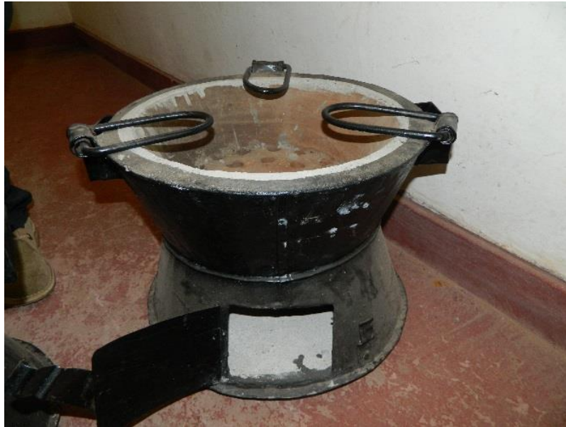
Plate 4.6: KCJ is a charcoal stove which was developed in 1983 by the Ministry of Energy. It has proved efficient with a potential to cut fuel requirements and easily portable. The ceramic liner is made of clay that is then cured and finally metal clads is fitted. (Source: Field Data, 2014)
