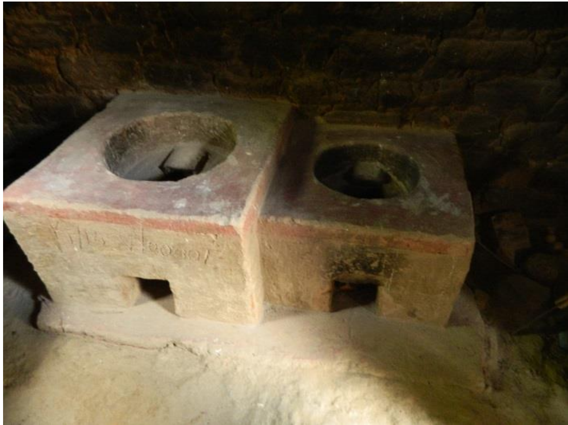
Plate 4.3: The Rocket Stove is a fixed model of firewood stove with two pot holders which makes it highly desired by rural households. The raw materials for construction include bricks, sand and cement. (Source: Field Data, 2014)
