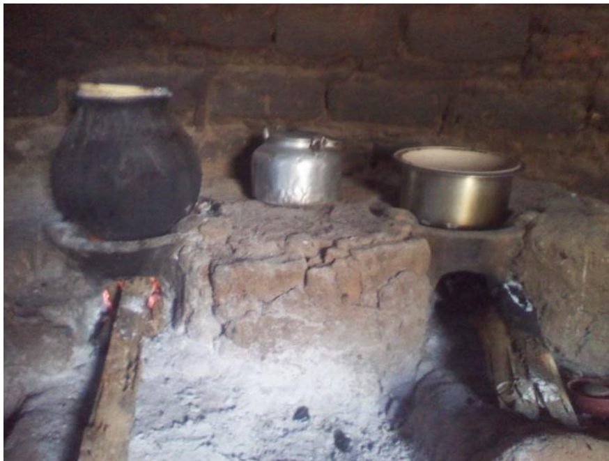
Plate 4.4: The fixed Maendeleo Stove is a firewood stove with two parts, a simple pottery cylinder with pot rests (known as the liner) that is built into a mud surround in the kitchen. Fuel is fed into the fire through an opening in the front of the stove, and it has no chimney, but it produces much less smoke than an open fire.
