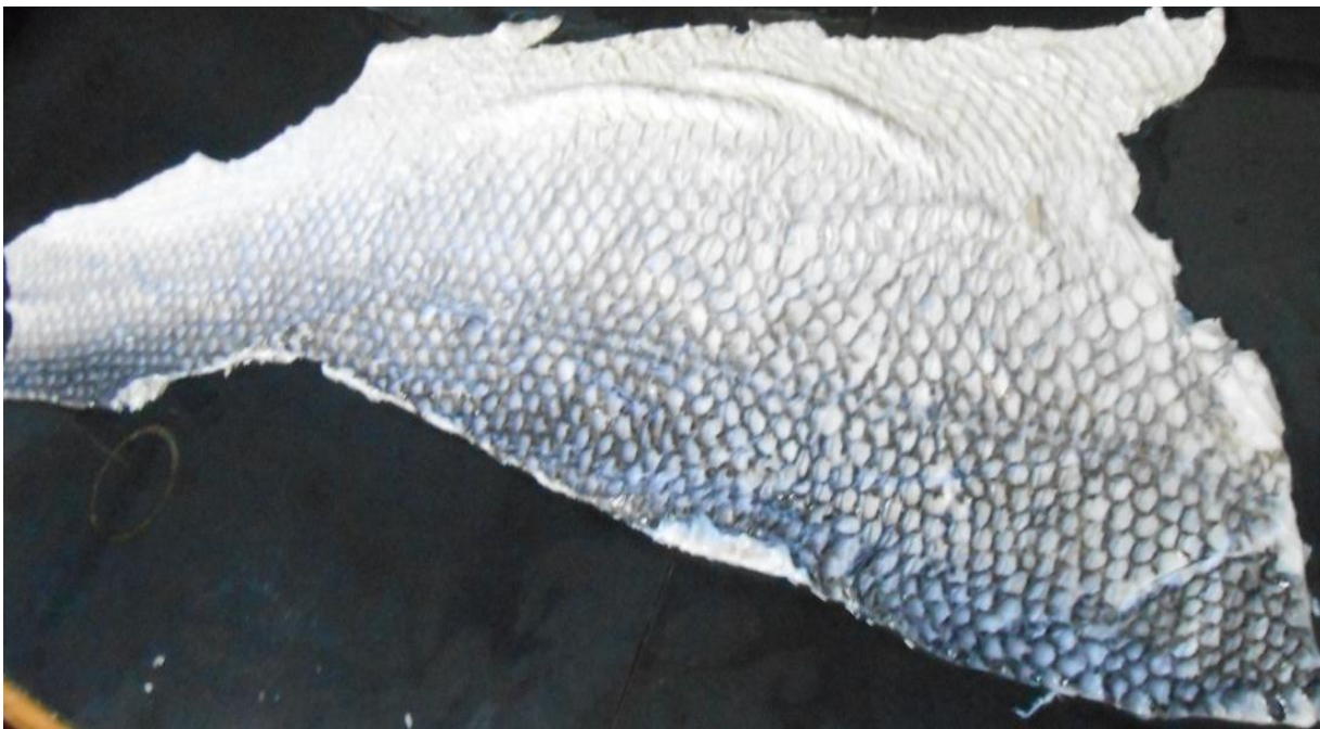
Figure. 4.20 b. Photograph of Nile perch skin ( Lates niloticus ) descaled within one hour using crude alkaline protease enzyme from Bacillus Cereus Strain 1-p
