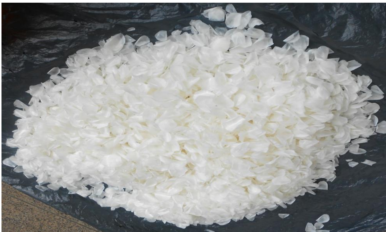
Figure. 4.21 Photograph of the recovered scales after descaling Nile perch skin using crude alkaline protease enzyme from Bacillus Cereus Strain 1-p .
