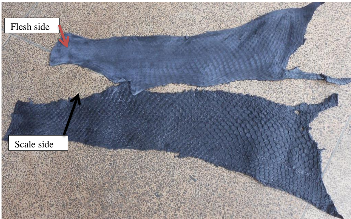
Figure 4.23b. Photograph of the resultant leather after post-tanning processing of Nile perch skin
