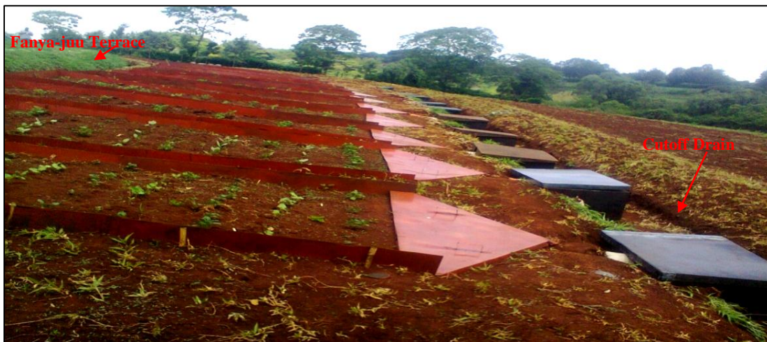
Plate 1.0: Plots installed at right angle to the contours and in between a terrace and a cutoff drain
