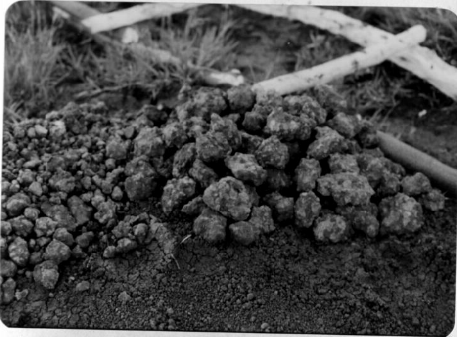
Fig.6.2: Pieces of the nodular cemented calcareous layer from well C3 in Kamleza scheme (Form III).
