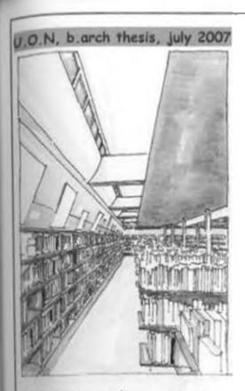
Fligh clerestory windows in an exterior wall, with a back reflecting surface to provide light on the vertical surfaces of the stacks at the wall, source http://www.librisdesign.org PSALI, this need would be satisfied with reduced sized windows, and the insufficient daylight would be supplemented by artificial means.
