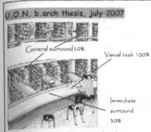
Recommended relative brightness of surfaces within the held of view for good visual comfort Taking 1000 as hightness for reading, mediate surrounding should be 305 while general surrounding should 108 source http://www.lbrisdesign.org
