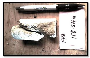
Plate A.2.8: Good brittle failure at approximately 45° to horizontal plane in muddy sandstones so UCS result was accepted
