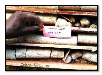
Plate A.1.3: Drill-core specimen in box from Comm. well at depth of 279.35 metres bgl; muddy sandstones
