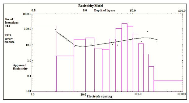
Figure C.1.1: Katz E-W drill-well auto-inversion resistivity model
