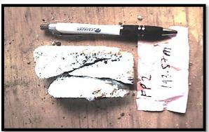
Plate A.2.7: Excellent brittle failure at approximately 45° to horizontal plane in muddy sandstones so UCS result was accepted
