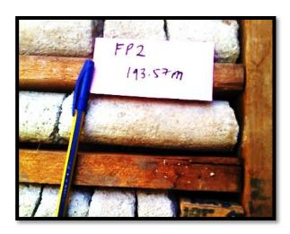
Plate A.1.7: Drill-core specimen in box from FP 2 at depth of 193.57 metres bgl; Muddy sandstones
