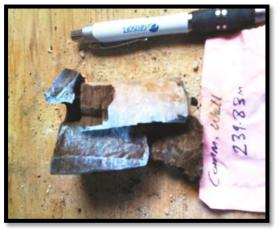
Plate A.2.2: Another display of brittle failure in muddy sandstones, so UCS result was accepted
