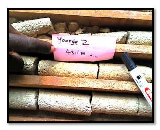
Plate A.1.11: Drill-core specimen in box from YO 2 at depth of 43.1 metres bgl; muddy sandstones
