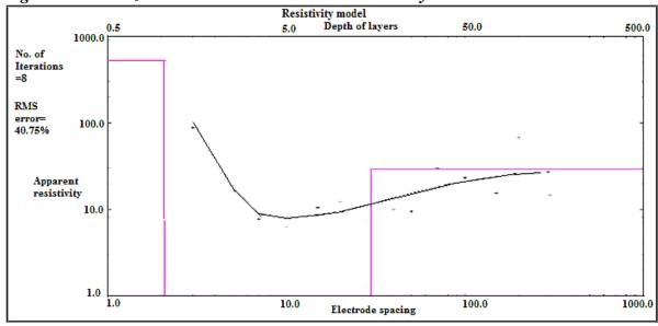
Figure C.1.2: Katz E-W drill-well forward model (user-provided parameters)
