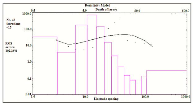
Figure C.1.7: YO 2 E-W drill-well auto-inversion resistivity model
