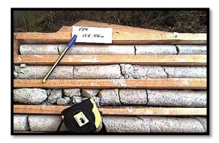
Plate A.1.8: Drill-core specimen in box from FP 3 at depth of 158.54 metres bgl; muddy sandstones
