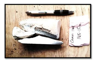
late 3.12: Coherent characteristic brittle failure in marlstones at about 45° to horizontal plane
