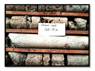
Plate A.1.2: Drill-core specimen in box from Comm. well at depth of 145.15 metres bgl; Marlstones
