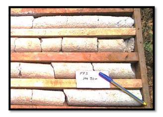
Plate A.1.6: Drill-core specimen in box from FP 2 at depth of 179.80 metres bgl; muddy sandstones
