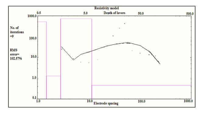
Figure C.1.8: YO 2 E-W drill-well forward model (user-provided parameters)
