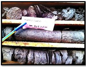
Plate A.1.4: Drill-core specimen in box from Katz. 3 at depth of 141.13 metres bgl; muddy sandstones
