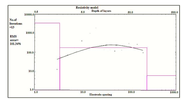
Figure C.1.4: FP 2 E-W drill-well forward model (user-provided parameters)
