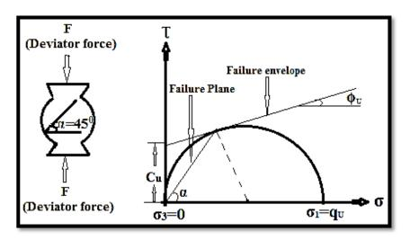
Figure 3.2: Schematic illustration of brittle failure at  $45^{0}$  during unconfined compression test (for  $\phi \approx 0$  and  $c - \phi$  soil) using a graph of shear stress verses normal stress, prepared from Mohr-Coulomb models in the internet
