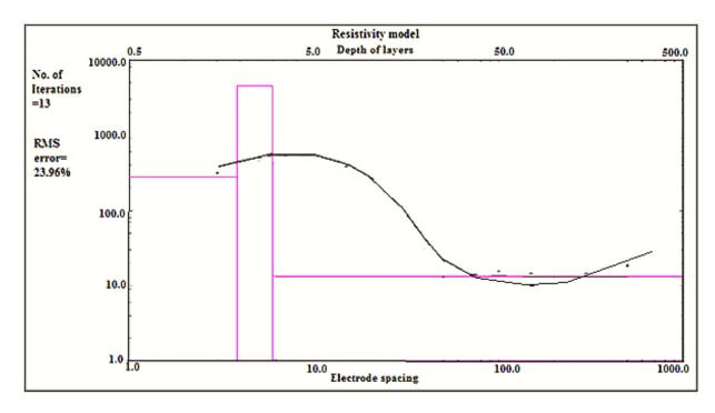
Figure C.1.6: FP 3 N-S drill-well forward model (user-provided parameters)
