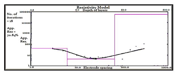
Figure 4.5: Comm. Well E-W drill-well' geo-electric forward model (user-provided parameters)
