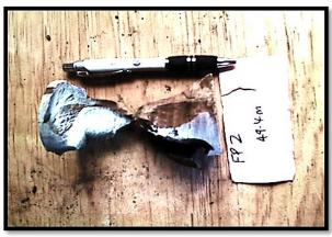
Plate A.2.9: Excellent brittle failure at approximately 45° to horizontal plane in muddy shales so UCS result was accepted
