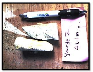
Plate A.2.11: Good brittle failure at approximately  $45^{\circ}$  to horizontal plane in muddy sandstones so UCS result was accepted
