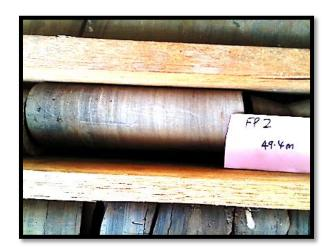
Plate A.1.5: Drill-core specimen in box from FP 2 at depth of 49.4 metres bgl; muddy shales
