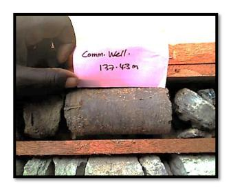
Plate A.1.1: Drill-core specimen in box from Comm. well at depth of 137.43 metres bgl; muddy sandstones
