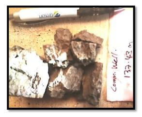
Plate A.2.1: Brittle failure, through crumbling, is at a vague approximate of 45° to horizontal plane, characteristic of muddy sandstones so UCS result was accepted, Ramamurthy and Sitharam (2010)
