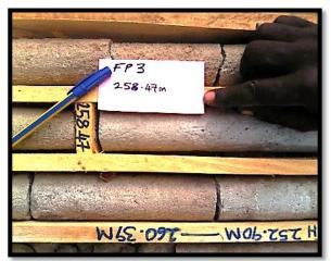
Plate A.1.9: Drill-core specimen in box from FP 3 at depth of 258.47 metres bgl; muddy sandstones
