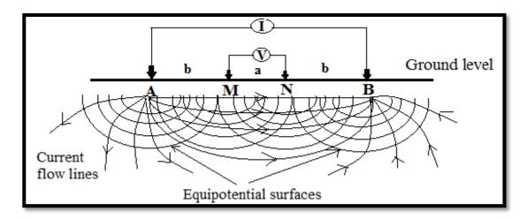
Figure 2.2: Representation of Resistivity parameters in Schlumberger configuration
