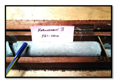
Plate 3.3: Core specimen in box from Katz. 3 at depth of 321.0 metres bgl, muddy sandstones
