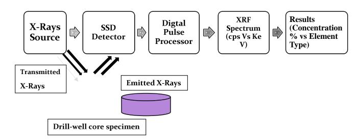
Figure 3.1: A schematic flow-chart to illustrate the principles of ED-XRF spectrometry
