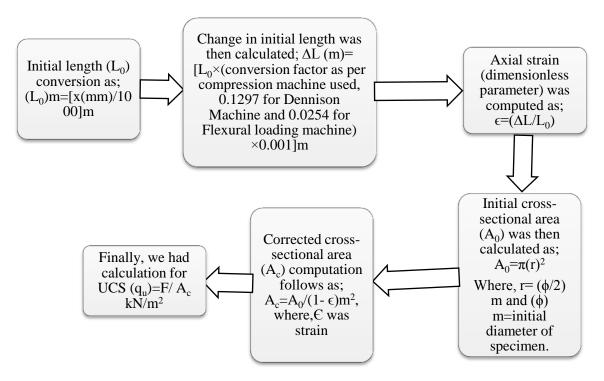
Figure 4.1: Flow-chart diagram illustration of steps undertaken in project analysis for UCSs
