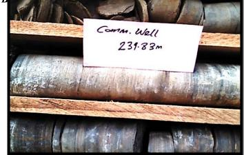
Plate 3.2: Drill-core Specimen in box from Comm. well at depth of 239.83 metres bgl, muddy shales
