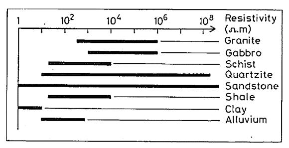
Figure C.1: Graphical representation for ranges for apparent resistivities for common rock types, after (Rahim, 2013)
