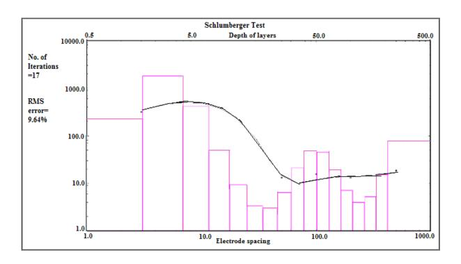
Figure C.1.5: FP 3 N-S drill-well auto-inversion resistivity model
