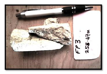
Plate 3.13: Excellent brittle failure at approximately 45° to horizontal plane in muddy sandstones so UCS result was accepted
