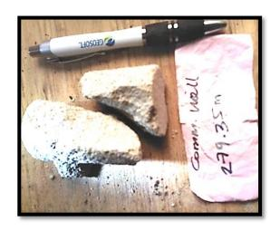
Plate A.2.3: Exhibition of brittle failure in muddy sandstones, so UCS result was accepted
