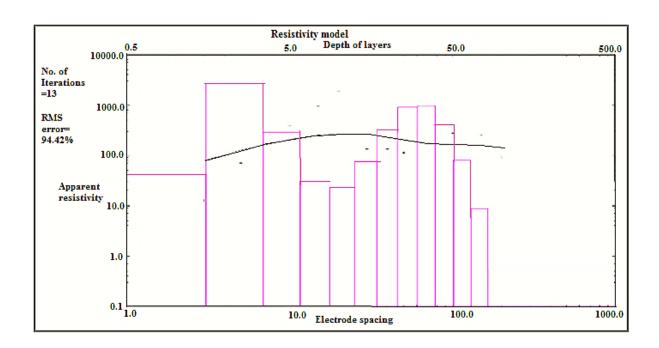
Figure C.1.3: FP 2 E-W drill-well auto-inversion resistivity model
