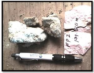
Plate A.2.6: Excellent brittle failure at approximately 45° to horizontal plane in muddy sandstones so UCS result was accepted
