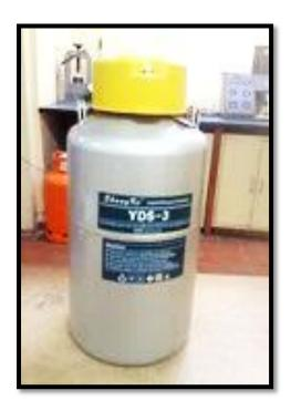
Plate 3.5: 'Giant' 3-litre thermos flask to hold liquid nitrogen
