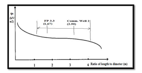
Figure 3.3: A schematic line-graph to illustrate the effects of varying specimens' length-to-diameter ratios verses UCS values and the range that is used in this this project, modified from (Lai & Olson, 2004)
