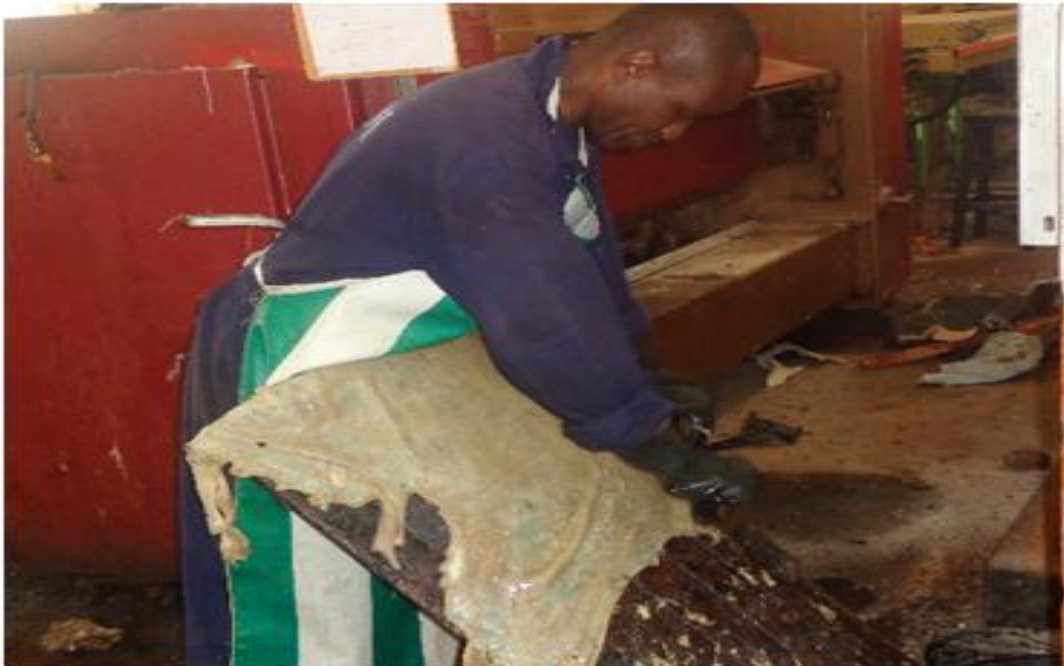
Plate 3.4: Fleshing operation to remove excess fat.
