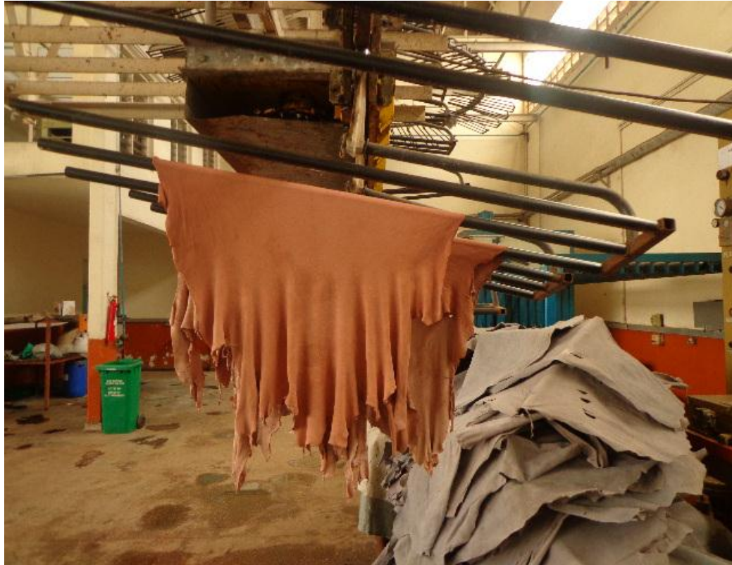
Plate 3.6: Hang drying of Mimosa tanned leathers
