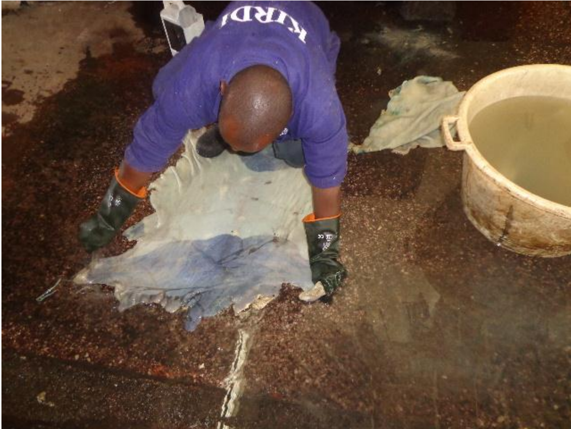
Plate 3.3: Scudding operation to remove hair roots and non- structural proteins.
