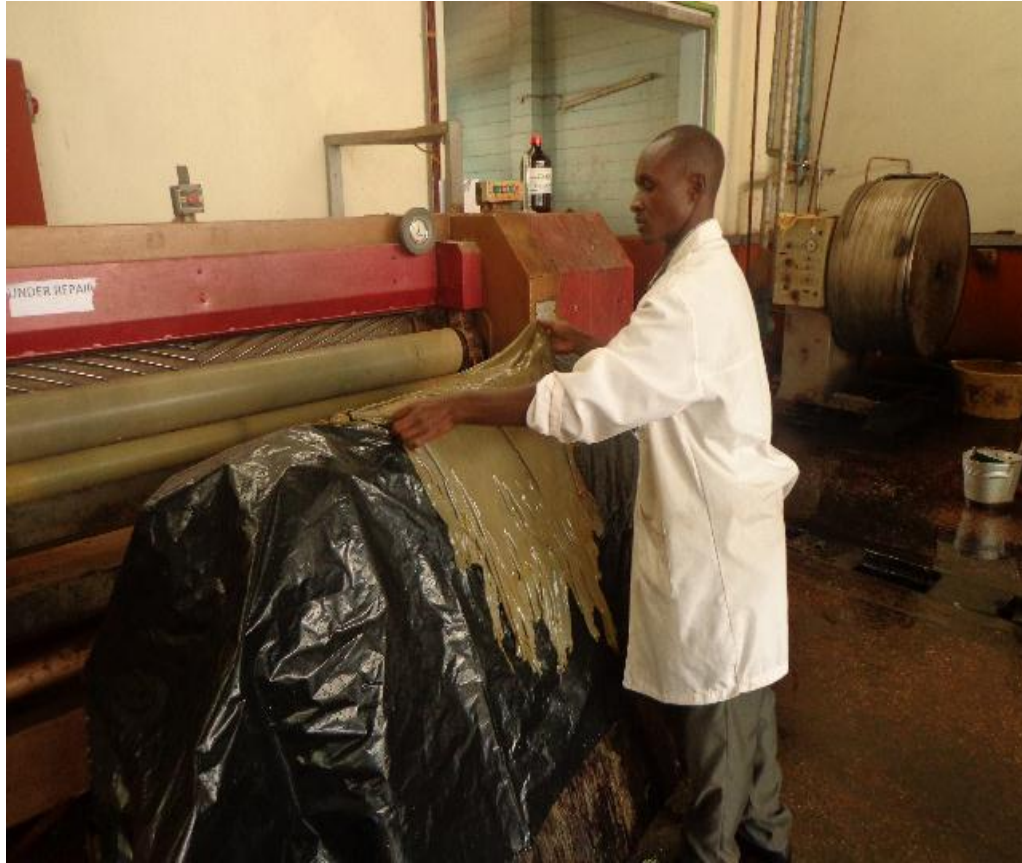
Plate 3.5: Horsing up of Plectranthus barbatus tanned leather to allow aging.
