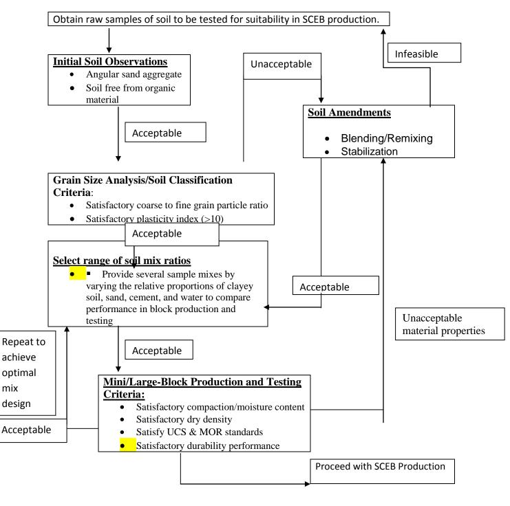
Figure 7 SCEB Testing Methodology
