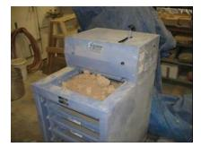
Figure 8, Gilson Testing Screen Model TS-1
