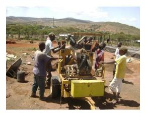
Figure 3, Mixing of soil and stabilizersFigure 4, Compressing &retrieving blocksPhotographs of workmen making CSEB- in Mavoko (source: author)
