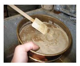
Figure 10 - #200 Sieve; mixing with water
