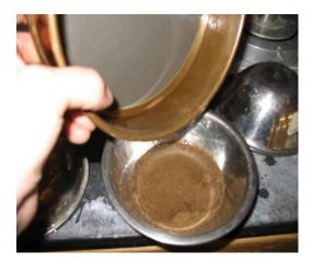
Figure 12 - #200 Sieve; Retained soil
