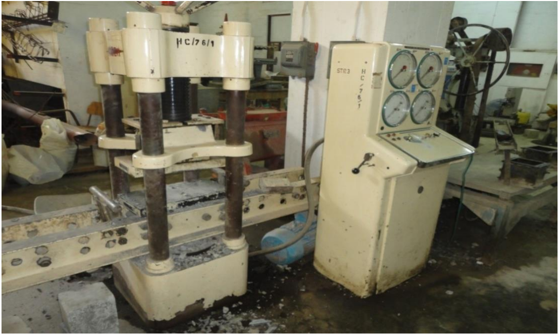
Figure 3.8: Picture of the Denison machine for testing concrete compressive strength
