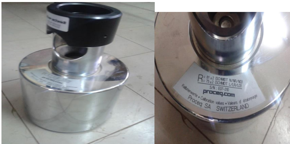
Figure 3.4: A picture showing a test anvil for periodic calibration of the Schmidt hammer
