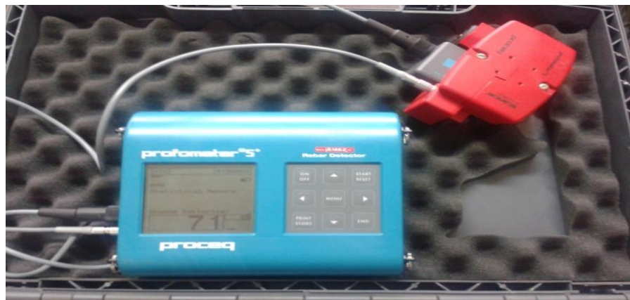
Figure 3.6: Picture of a Profometer 5+ covermeter
