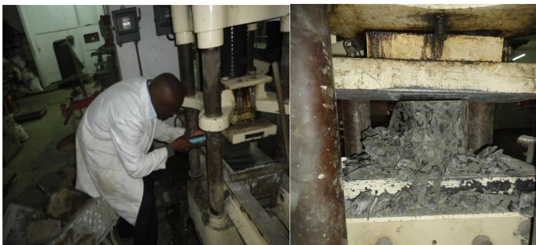
Figure 3.7: Taking the Rebound measurements before loading the cubes to failure
