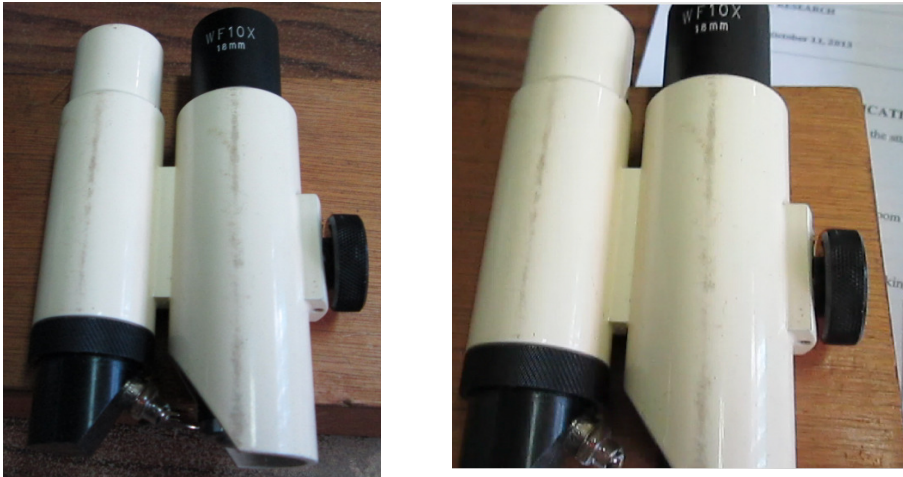
Fig 3.1 Crack width Gauge used to measure cracks width
