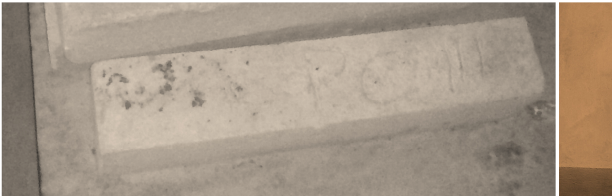
Photo A2-2: Beams cast for flexural testing
