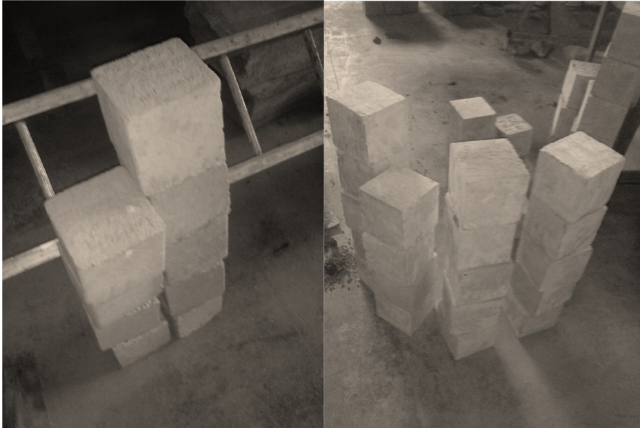
Photo A2-1: Cubes tested with the crushing strength machine
